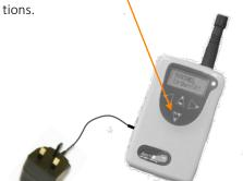
(Charger can be left permanently connected or it can boost charge from empty in 8 hours)
