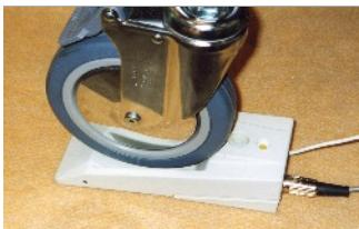
The bed/chair leg is positioned in the recess of the wedge. For beds it is recommended to use a leg near the headboard which carries greater patient weight.
