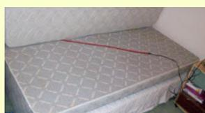
**P143G Bed Ribbon Sensor** performs like the Bed Mat, but has the advantage of fitting underneath the mattress. The unit may not work for restless sleepers as it may trigger at the bed extremities. It may also not work with some bed/mattress combinations depending on the weight of the user.
