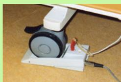
and beds and will activate an alarm condition when the bed is vacated.
